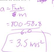
14. What force is needed to accelerate a 60.0 kg cart and rider from rest to 4.2 m/s in 2.5 seconds when the friction force is 24 N?
