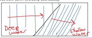
Waves traveling perpendicular to the new medium ( $\Theta_i = 0^\circ$ ) continue in the same direction.
