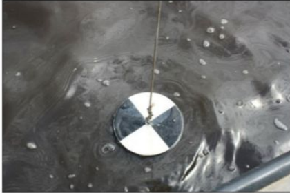
Figure 3. Secchi disk being lowered into water to measure clarity. ( https://www.flickr.com/photos/usace_albuquerque/5999717664 )
